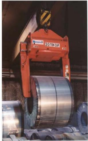
Combining operating efficiency, protection of the coil, and utilization of the overhead crane system, the standard M5067 coil grab offers the most comprehensive coil handling features. The lifter can be operated with cab, pendant or remote controls. Standard units in 10 to 50 ton
