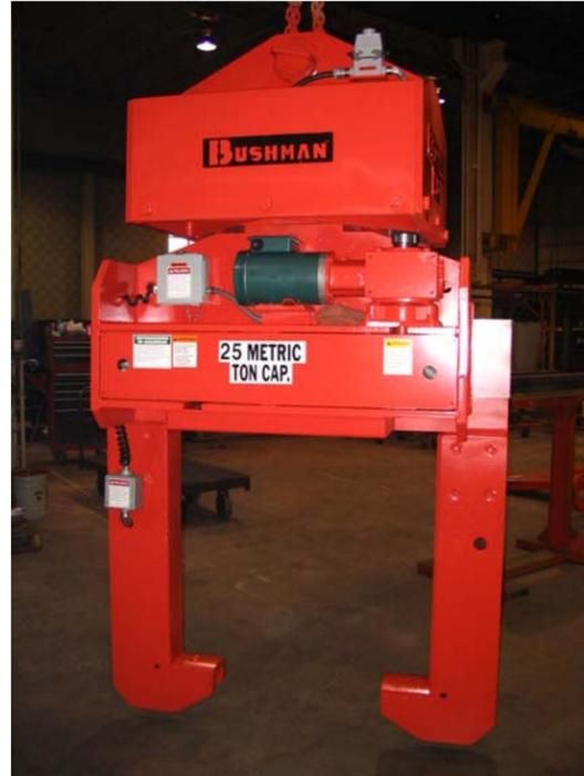
The MR5067 coil grab from Bushman AvonTec is a low headroom lifter designed to give precise coil positioning. A gear motor accomplishes rotation with an integral pinion driving a geared bearing that is mounted in compression. An overload clutch protects the rotation drive from shock loading.
