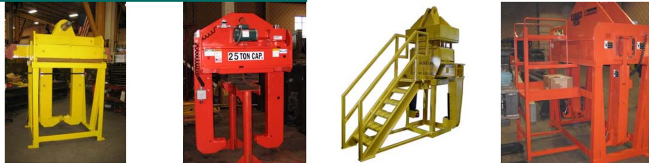
Coil lifters are large and top-heavy. They can be designed for storage only or as a full maintenance platform. When not in use, each coil grab should be stored on a stand designed for its specific size and weight.
