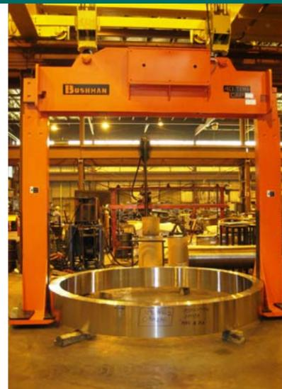
This customer needed a faster and safer way to lift forged rings into and out of their vertical turret lathes. They were lifting them manually using three chains that had to be carefully rigged and adjusted. This customer-
