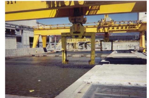
These two 31-ton coil grabs are used with fully automated cranes over an outdoor coil quenching pool.
