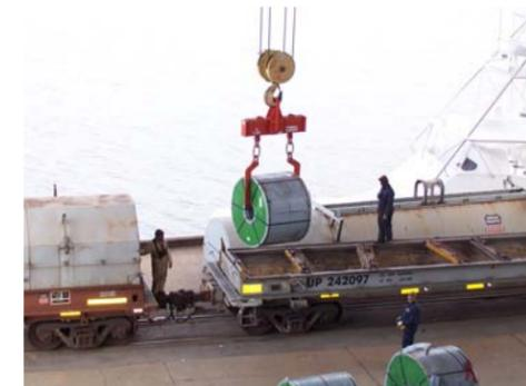
This 25-ton capacity adjustable coil lifter is offloading steel coils from a railroad car in Houston.
