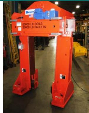
This combination horizontal pallet lifter can lift 30-ton coils in eye-horizontal position or 15-ton coils lying eye-vertically on a pallet.
