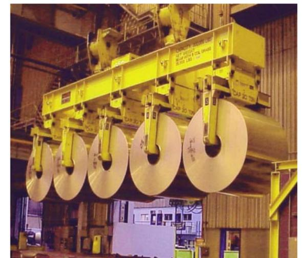
This single spreader beam simultaneously supports five coil grabs that each lifts a 20-ton aluminum coil.
