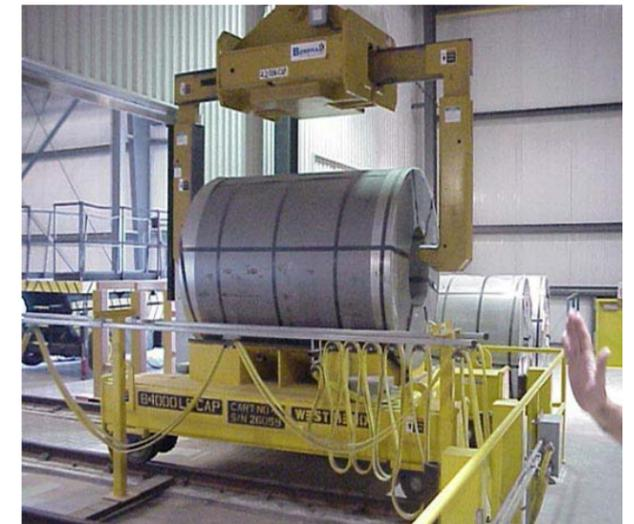
One of two 42-ton coil grabs on fully automated coil storage cranes loading a coil on a transfer car.
