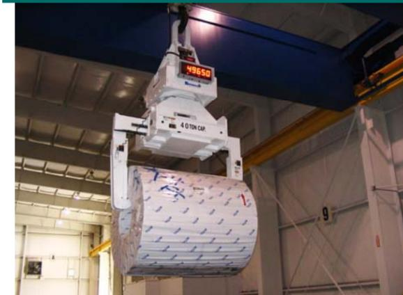
Bushman AvonTec coil lifters can be equipped with weighing systems to weigh coils during the lift. This saves time by not having to use a separate floor scale.
